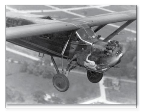
One of the Hunter brothers made some adjustments to the Wright Whirlwind engine that carried their plane, the City of Chicago, through a successful record breaking endurance flight in 1931. Manufacturers' Aircraft Association Records.
