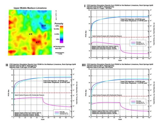
**Figure 4.** Numerical simulations of three  $CO_2$  injection scenarios representing three different locations within the best reservoir interval in the Madison Limestone: the Upper Middle Madison.
