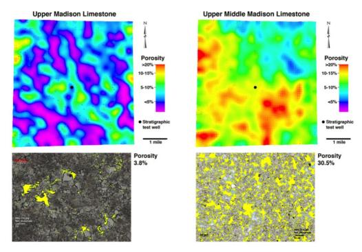
**Figure 3.** The upper two diagrams represent stratal slices through the Upper and Middle Madison Limestone showing the variability of reservoir properties within the formation. The lower two diagrams are thin section photographs and illustrate the extreme differences in porosity within the Madison Limestone.
