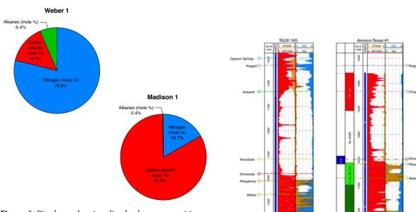
**Figure 6.** Pie charts showing dissolved gas composition of the Weber and Madison Formation fluids (above). The substantial differences in composition suggest that the Madison and Weber formation fluids are not in communication. Fluid inclusion compositions for wells from the Moxa Arch and Rock Springs Uplift (right; from Campbell-Stone et al. (2010)). In both cases, the Triassic units have acted as hydrocarbon seals above the Madison and Weber formations.
