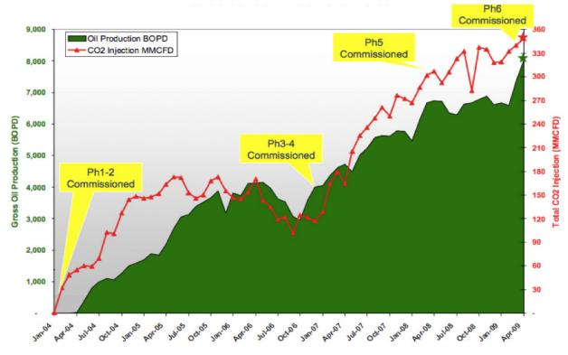
Figure 12. Example of CO<sub>2</sub> flooding and stranded oil recovery at the Salt Creek Oil Field.
