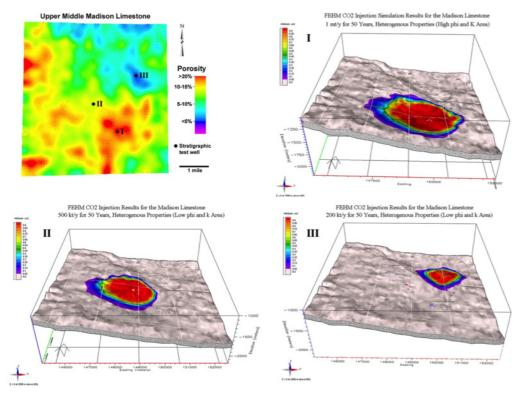
**Figure 9.** Diagram showing the size of the  $CO_2$  plume resulting from  $CO_2$  injection into the Madison Limestone from  $CO_2$  injection at three locations in the study area (shown in upper left panel).
