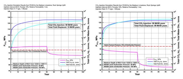
**Figure 8.** Output from numerical simulations of two  $CO_2$  injection scenarios. The left panel shows a scenario in which only a small amount of formation fluid is produced during  $CO_2$  injection, while the right panel shows a scenario in which the volume of formation fluid produced equals the volume of  $CO_2$  injected (1:1 ratio). Note that in the left panel,  $CO_2$  injection causes the pressure to rapidly approach fracture pressure.
