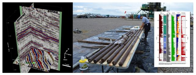
**Figure 2.** From left to right, this figure shows results from the 3-D seismic survey, core from the stratigraphic test well, and a well log suite from the WY-CUSP study site at the Rock Springs Uplift.
