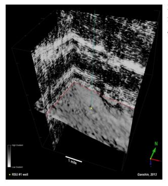
**Figure 7.** Vertical sections and stratal slice through the 3-D seismic volume. The homogenous nature of the Upper Madison suggests that this interval has continuous confining integrity.
