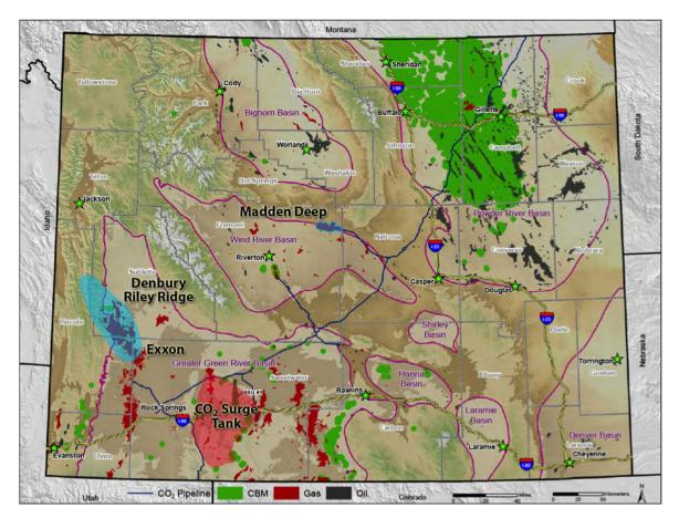
**Figure 11.** Map showing the location of the EOR targets (black), CO<sub>2</sub> pipelines (blue), CO<sub>2</sub> production sites (blue), and position of the Rock Springs Uplift as a regional surge tank for CO<sub>2</sub> and EOR projects.
