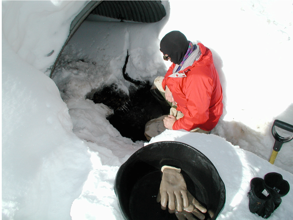
Figure 4. Streamflow measurement using a bucket at a culvert on Middle Fork Rock Creek, site MB-4, February 12, 2002.
