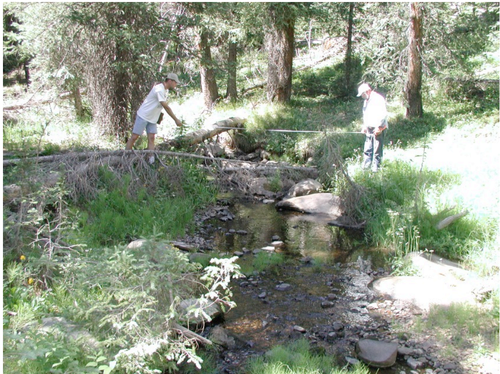
Figure 3. Measurement of channel width on unnamed tributary to Fish Creek, site BC-5, July 15, 2002.
