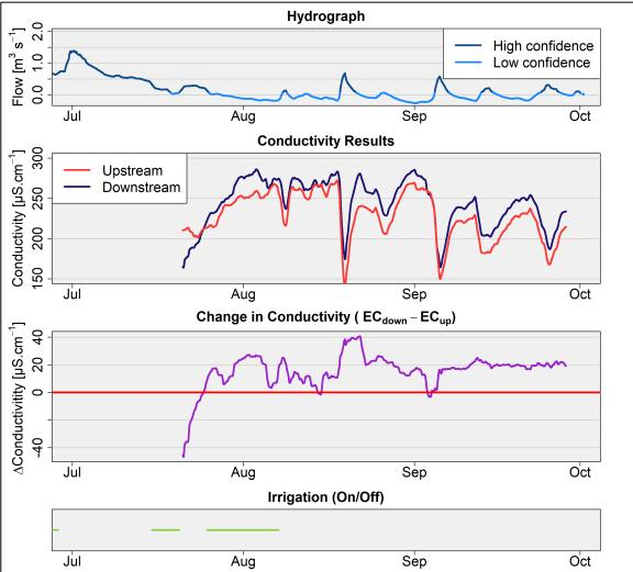
Figure 11: Conductivity analysis using the upstream and downstream conductivity loggers. Return flow signal becomes apparent through the reach analysis.
