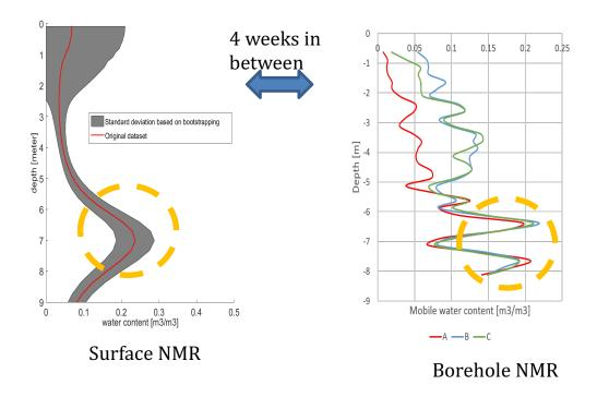
Figure 8. Comparison of results from surface NMR and time- borehole NMR showing water content increasing at the same depth in the subsurface.
