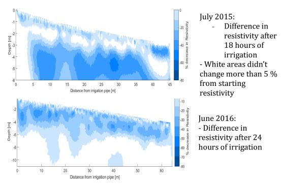
Figure 7. Comparison of time-lapse resistivity during irrigation experiments in 2015 and 2016. The changes in resistivity are being converted to changes in water content.
