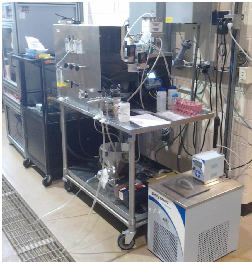
Figure 3: The NF test-apparatus, showing the conical reservoir below, the instrumentation above, and the NF membrane cell in white (with blue lettering) at the very top.
