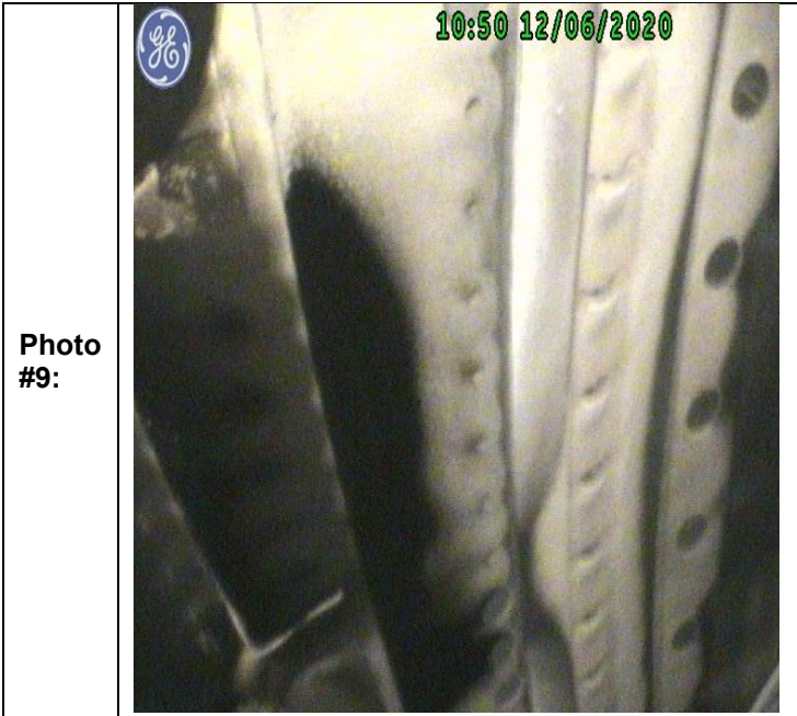
Photo #9: Louvered cooling ring: Acceptable.
