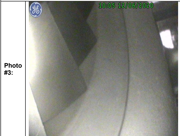
1 st Stage Compressor Blades: Acceptable
