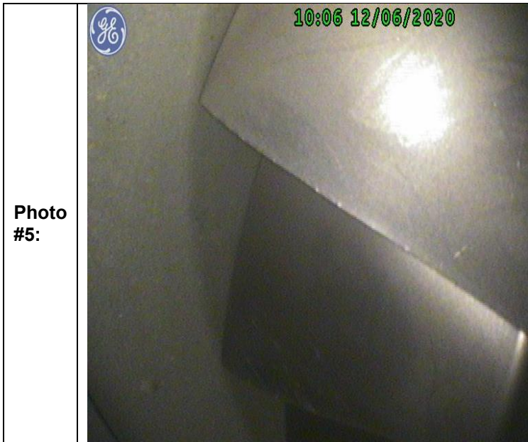
1 st Stage Compressor Blades: Acceptable
