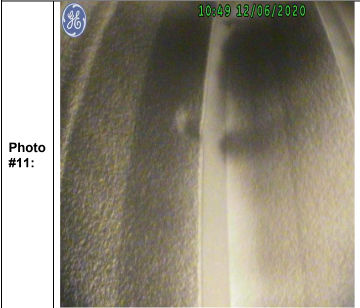
Photo #11: Combustion liner cooling rings: Acceptable
