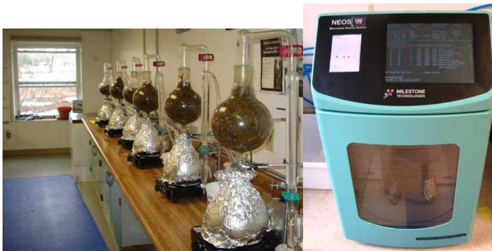
Figure 1. Steam distillation (left) of mint from container experiments at ShREC. Solvent-free microwave extraction labstation (right) at ShREC.
