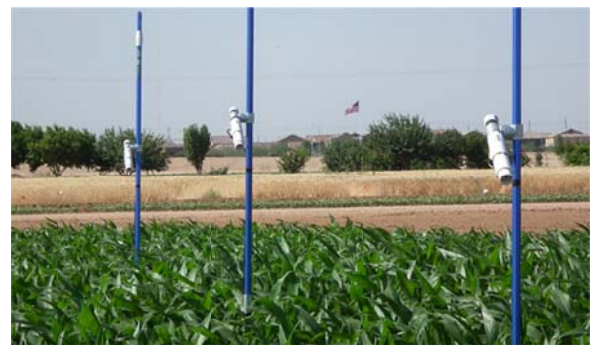
Figure 1. Deployment of infrared (IR) thermometers in the experiment conducted at the USDA-ARS research center in Maricopa, Arizona.
