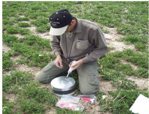
Figure 2. Gas chambers established in irrigated field and measurement of trace gases
