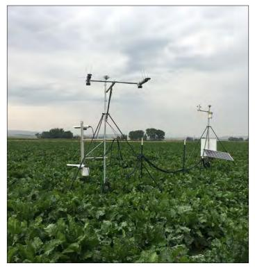
**Figure 1**. The Bowen energy balance system in a developed sugarbeet field at PREC.
