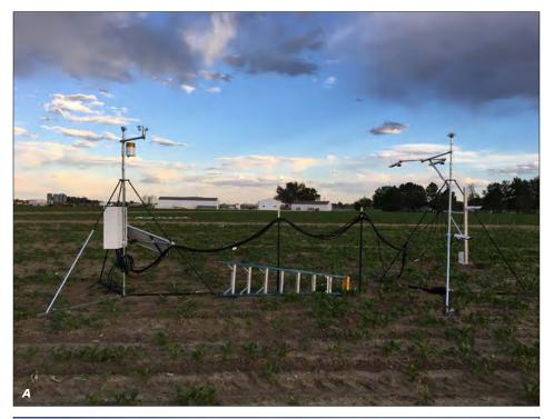
**Figure 2**. Bowen ratio-energy balance system for measuring crop evapotranspiration and crop coefficients during the growing season (A); and for measuring evaporative losses during the nongrowing season (B).
