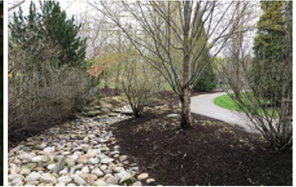
Stormwater Element – break down scale of boulders and use as a surface in stormwater BMPs and swales
