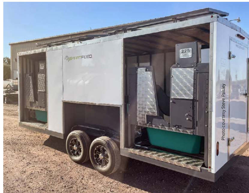
SAREC's new C-lock supplement feeders are self-contained units powered by solar panels and managed via cellular signal.
