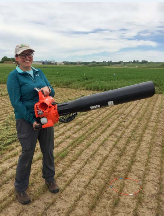
Grad student Samantha Nobes (M.S., 2021) vacuums sample insects in a recently harvested experimental plot at SAREC using a modified leaf blower.
