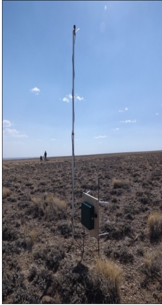
Figure 3. SM2BAT+ device deployed to record bird and bat calls.
