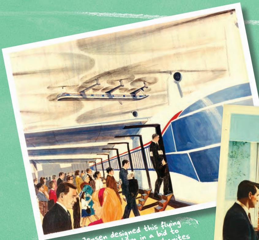
Martin Jensen designed this flying mass transit system in a bid to transport Los Angeles suburbanites to the center of the city. The competition was a subway train. The flying transit car had ten rotors and jets driving the rotors. Designed to hold 100 passengers, the car had seven entrance doors and seven exit doors on the opposite side. Jensen's design lost the competition. Martin Jensen Papers.
