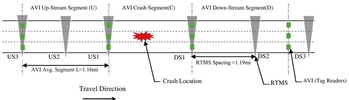
Fig. 1. Arrangement of RTMS and AVI segments.
