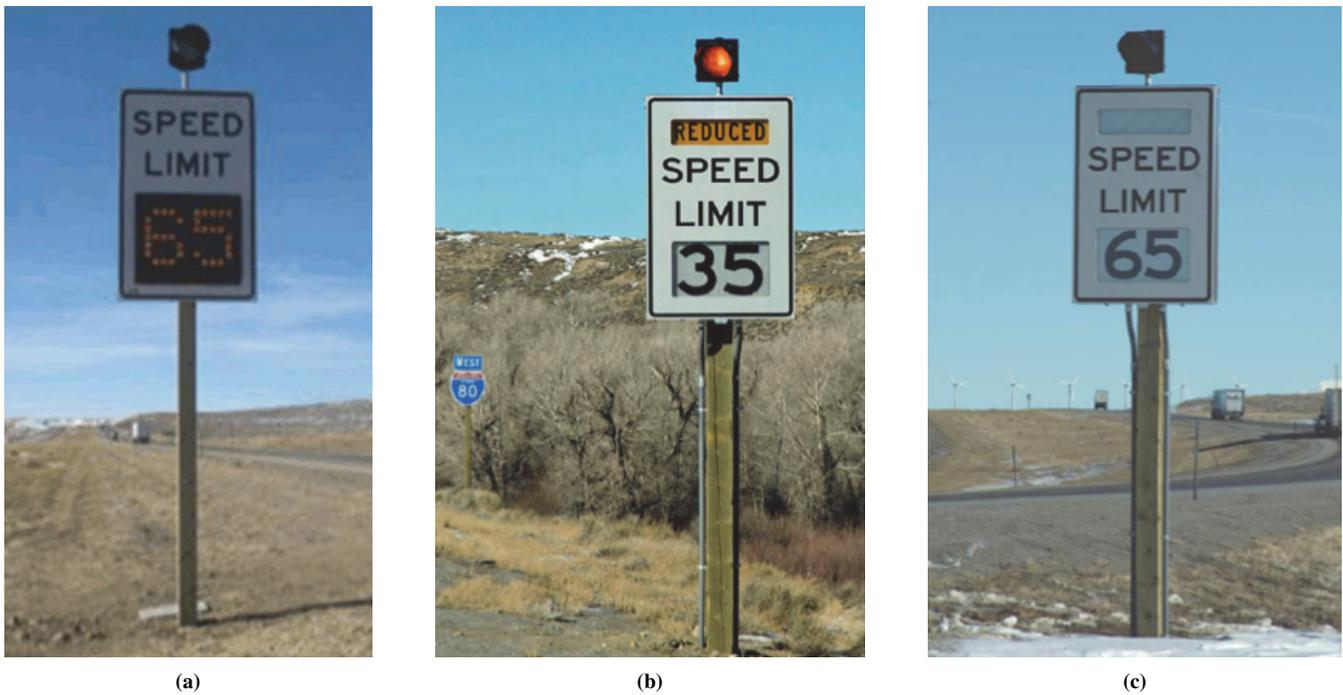
FIGURE 1 Typical VSL signs with flashing beacon: (a) LED and (b and c) scrolling film.
