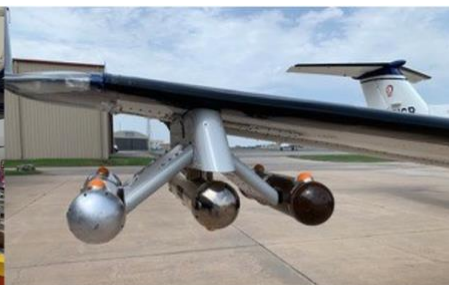
Here, acceleration meters are installed on the PMS-style canisters to determine flutter during test flights.
