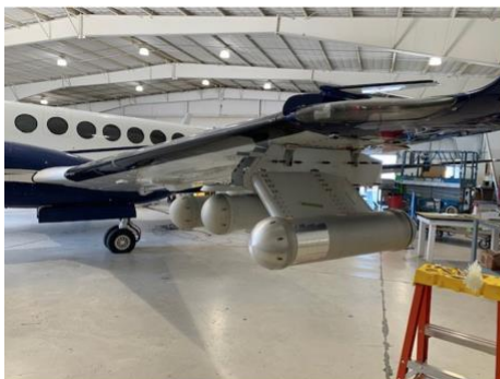
Wing pylons and canisters
