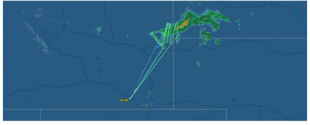
Picked up some icing in the clouds. Last run at 13k', the ice on the wings was rough, and formed on the aft edge of the boots. We descended to 11k' which melted the ice off. Returned to Laramie at 11k'..
