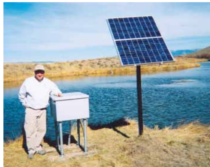
Bill Nye with a solar-powered aerator. Aeration increases oxygen levels and speeds up the breakdown of organic material in a pond.
