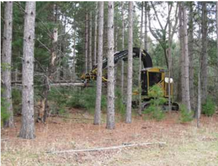
Mechanical harvesting systems, such as this whole tree processor, are light on the land and very efficient at thinning conifer stands.
