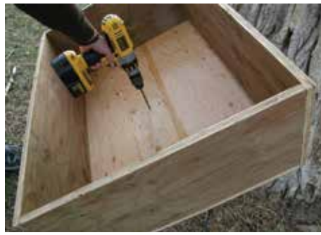
Holes in the bottom allow collection of "worm tea" – the juices secreted and used for liquid plant fertilizer.
