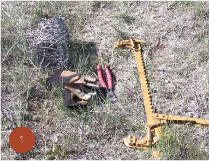
A roll of barbwire, fencing pliers, fence stretcher, and leather gloves are commonly used to repair fence. These can be purchased at most farm and ranch supply stores or feed stores.
