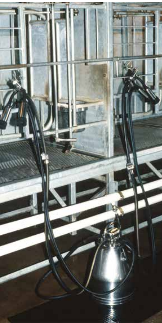
Bucket milker assembled for two goats. Milking machines allow a single person to milk multiple animals at once but increase cleaning time.
