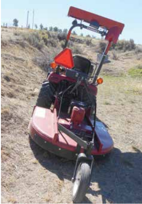
The narrow wheelbase of compact tractors increases the danger of tipping while working on slopes.
