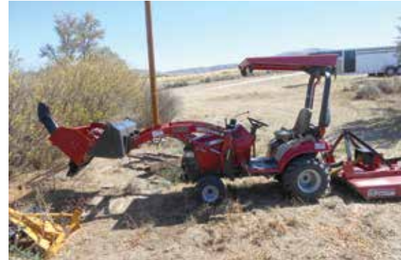
Some of the implements available for compact tractors. The weight of these implements should be considered when operating the tractor.
