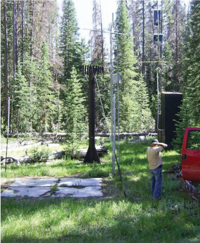
Seasonal scenes of the Whiskey Park SNOTEL site (elevation 8,950 feet) on the Wyoming-Colorado border. Note snow pillows in the photograph on the left.
