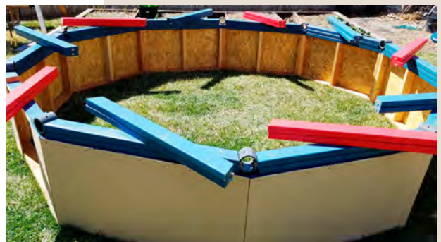
An exploded view of several 2 x 4 struts with hanger bolts and the dome connectors.
