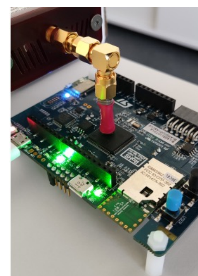
Figure 1: EMFI attack on a STM32 Discovery Board
