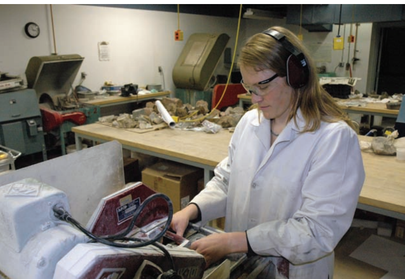
Photo: University of Wyoming geology graduate student Karri Sicard uses a diamond-tipped trim saw to prepare a schist for microscopic examination of minerals contained within a rock sample. UW is taking steps to elevate graduate education to a higher level of prominence among university priorities. (UW Photo)
