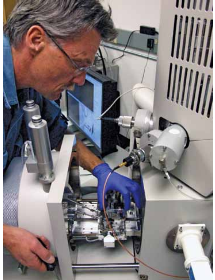
Laboratory Technician Norbert Swoboda-Colberg places a sample into the new Field Emission Scanning Electron Microscope.
