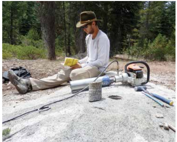
University of Wyoming researcher Jesse Hahm used a gas-powered drill to sample cores of fresh bedrock for geochemical analysis. He is the lead author of a study that shows how bedrock influences forests and landscape evolution much more than was previously thought. (Claire Lukens Photo)
