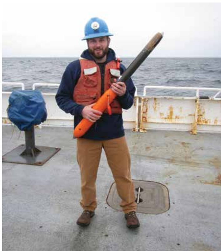
Will Fortin, a UW doctoral student in geology and geophysics, participated in a Chief Scientist Training workshop funded by the National Science Foundation and the Office of Naval Research. Here, he holds an instrument called a uCTD that can provide salinity, temperature and depth readings of the ocean. (Gordy Stephenson Photo)
