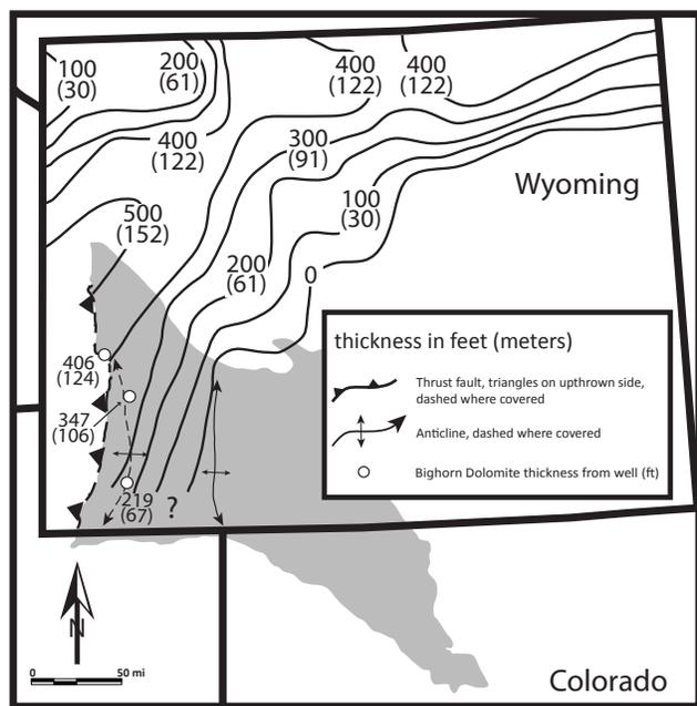
**Figure 4.** Isopach map of the Bighorn Dolomite in Wyoming. Circles indicate thickness of Bighorn Dolomite as interpreted from well logs; the Greater Green River Basin is highlighted in gray; the front of the Sevier fold-and-thrust belt, Moxa Arch, and Rock Springs Uplift are represented with map symbols (see Fig. 1). Modified from Peterson (1989).
