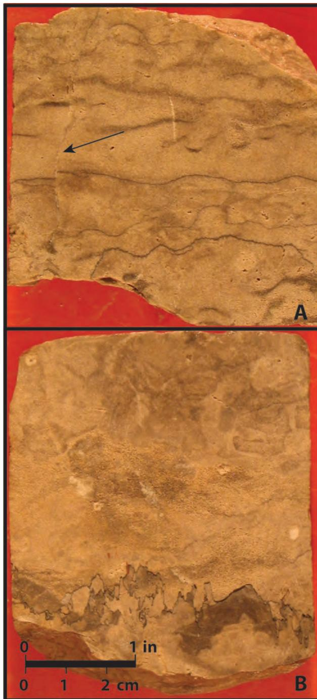
**Figure 6.** Bighorn Dolomite core photograph showing structural and compaction heterogeneities. **A**, Small calcite-filled fracture with mm-scale offset (arrow). **B**, Well-developed stylolite near base of core with high porosity zone above stylolite and low porosity below stylolite.
