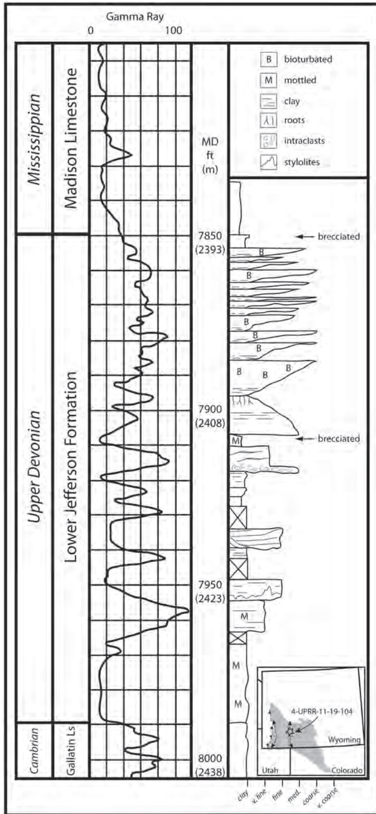
**Figure 9.** Lower Member of the Jefferson Formation core correlated with gamma ray log from the 4-UPRR-11-19-104 well, located on the Rock Springs Uplift (see inset map). Birdbear Member of Jefferson Formation and Three Forks were removed by pre-Mississippian erosion. A clastic horizontal scale was chosen for the core description because of the profusion of well-rounded quartz grains.
