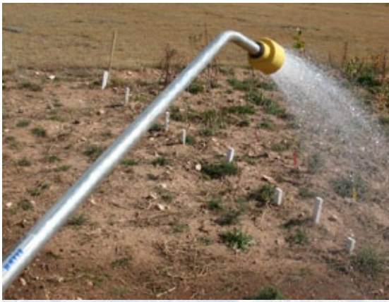
Breakers on extension handles work well for hard-to-reach areas.
