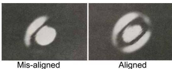
In case the beam spot escapes from the center of the fluorescent screen after correction, bring it to the center by manipulating the GUN HORIZ knobs.
