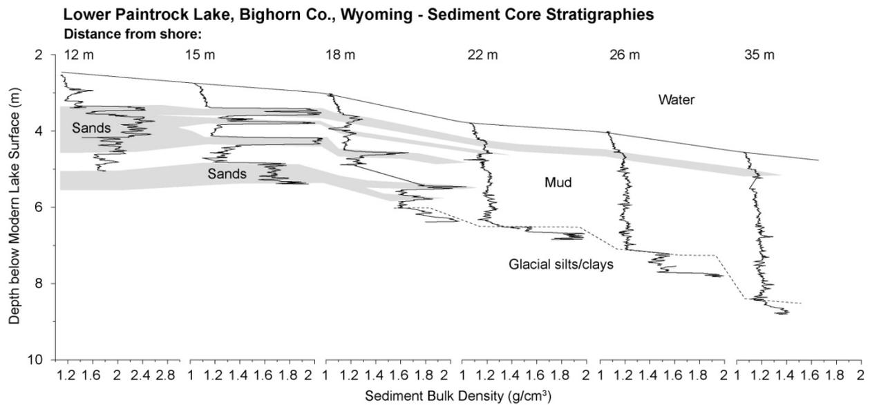
Figure 1. Sediment characteristics (such as sediment density above) in a transect of sediment cores collected perpendicular to shore can be used to track shifts in a lake's shoreline over time. Here, cores collected in July 2010 from Lower Paintrock Lake show layers of sand associated with periods of low water when the shoreline moved toward the lake center.
