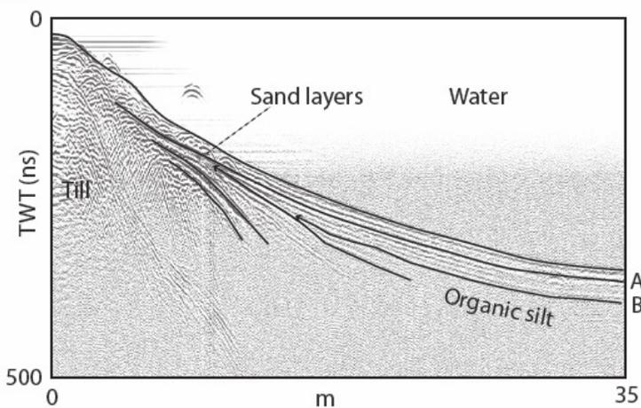
Figure 2. Ground-penetrating radar profiles show submerged paleoshorelines (sand layers marked by the convergence of stratigraphic layers and large amplitude radar reflections) in Lower Paintrock Lake. This profile spans the area of core locations (see Fig. 1), and confirms that the sand layers in the cores are associated with episodes of near-shore erosion (truncation of off-shore layers, such as layer B, at arrows). Data are presented in
