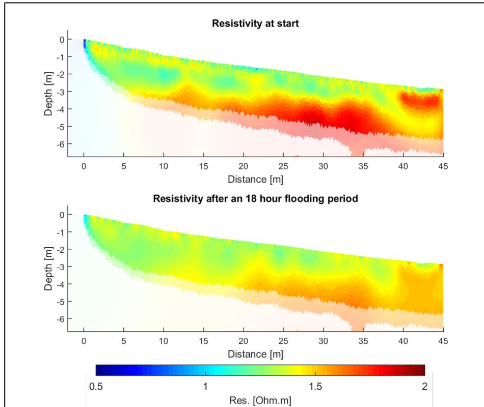
Figure 6. Time Lapse ERT during wetting and drying (before, during and after irrigation applications).
