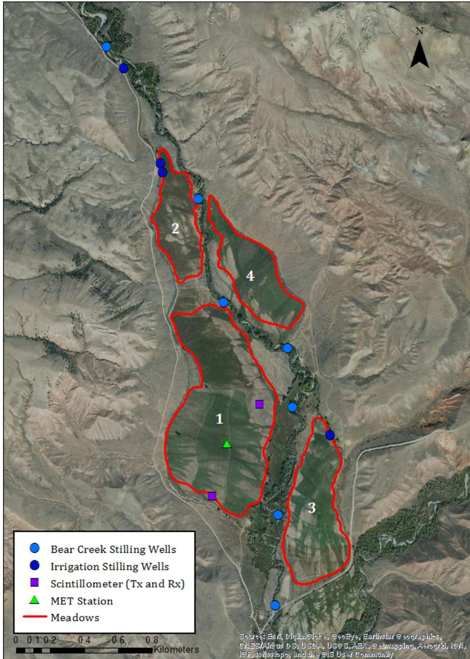
Figure 2. Location of installed instrumentation relative to irrigated meadows and stream.
