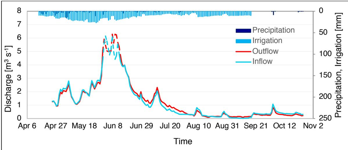
Figure 4. Inflow and outflow hydrographs used to calculate return flow in 2015 ( $Q_{RT}$ ).
