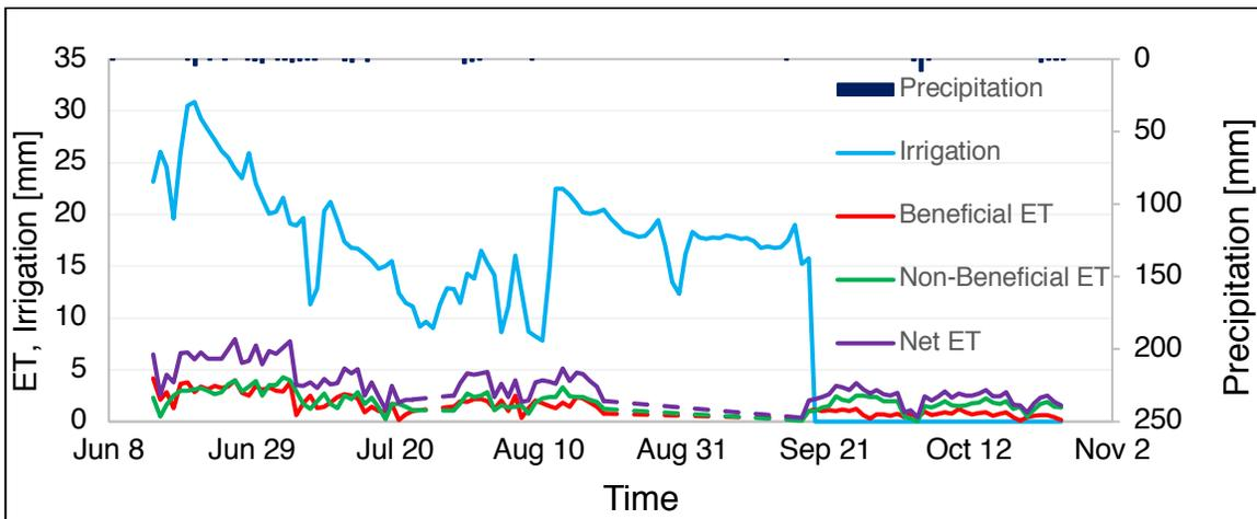
Figure 5. Evapotranspiration for the 2015 irrigation season. Non-beneficial ET is the evapotranspiration for the riparian areas calculated from using Penman-Monteith. Beneficial ET was calculated from the scintillometer.
