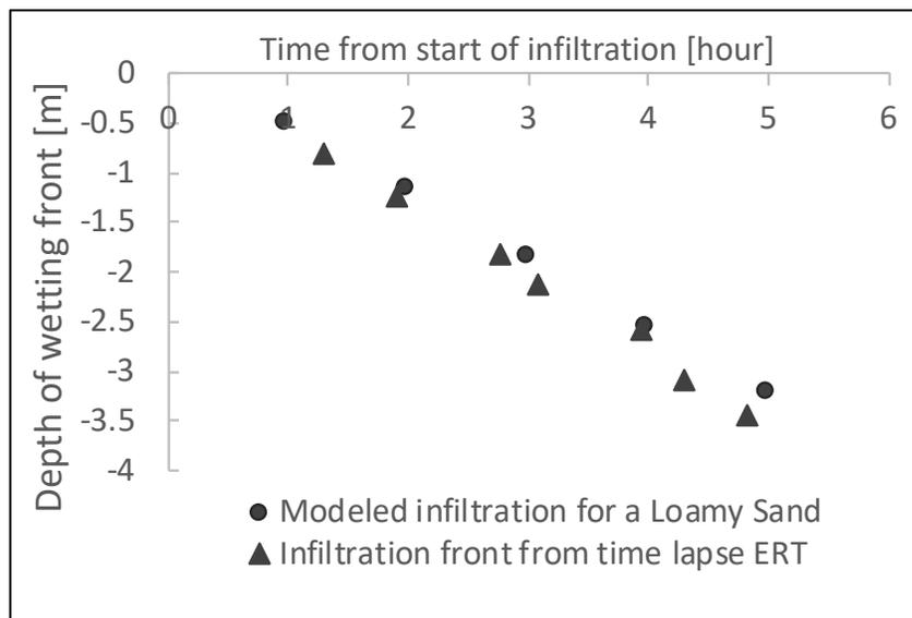
Figure 10. Comparison of modeled and observed wetting front movement in the subsurface under intense irrigation.
