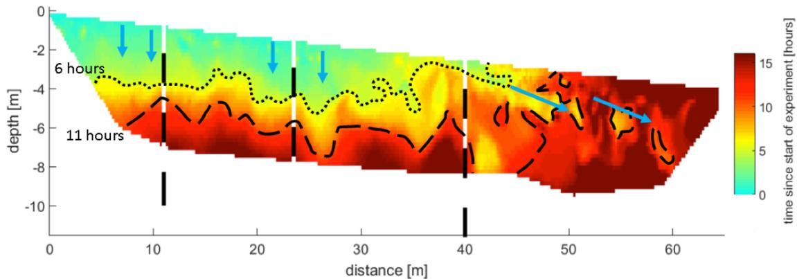
Figure 9. Wetting front velocities and dominant flow paths identified from the time-lapse ERT data.
