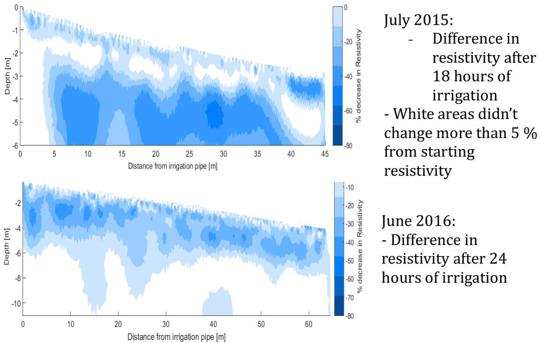
Figure 7. Comparison of time-lapse resistivity during irrigation experiments in 2015 and 2016. The changes in resistivity are being converted to changes in water content.
