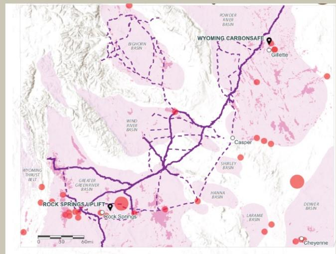
▲ A preliminary figure from the PCOR CO<sub>2</sub> Atlas showing Wyoming’s CO<sub>2</sub> sources, infrastructure, and formations and basins capable of sequestration.
