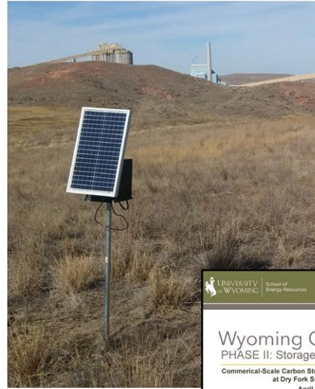
▲ A fully deployed CO<sub>2</sub> sensor station
