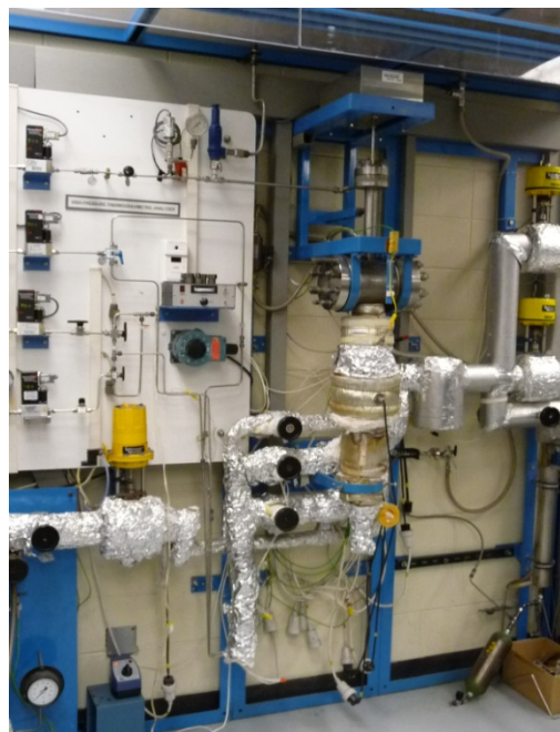
Figure ES-5. Photograph of the Bench-scale U-GAS® Gasifier Used in the Testing.
