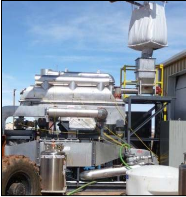
Figure ES-3 Mobile WRITECoal™ 1-2 MW th -Scale Pilot Plant at WRI to be integrated with the Oxy-Combustion System at SRI. Blue item is condenser/heat exchanger.
