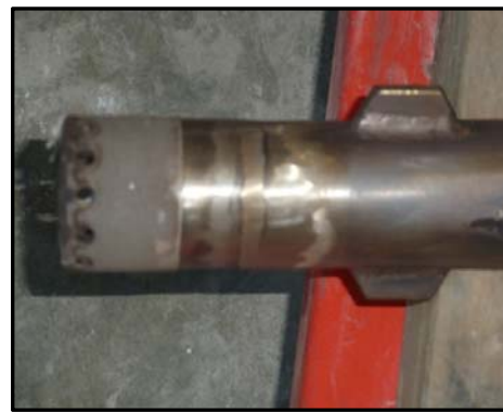
Figure ES-4 Photograph of the F/W Oxy-Burner Tip after Testing at SRI (above)
