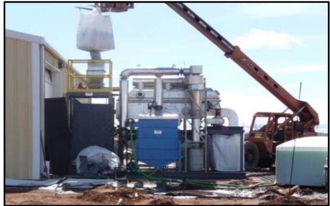
Figure ES-3 Mobile WRITECoal™ 1-2 MW th -Scale Pilot Plant at WRI to be integrated with the Oxy-Combustion System at SRI. Blue item is condenser/heat exchanger.
