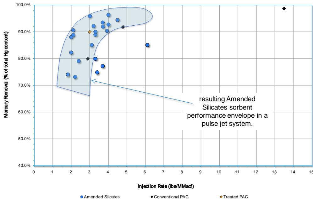
**Figure 3. Mercury removal as a function of sorbent injection rate for baghouse plant configuration**
