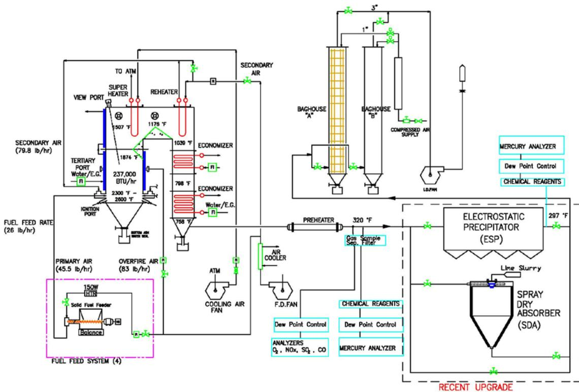
**Figure 1. Schematic of the Coal Combustion Test Facility with the ESP and the SDA (Recent Upgrades)**
