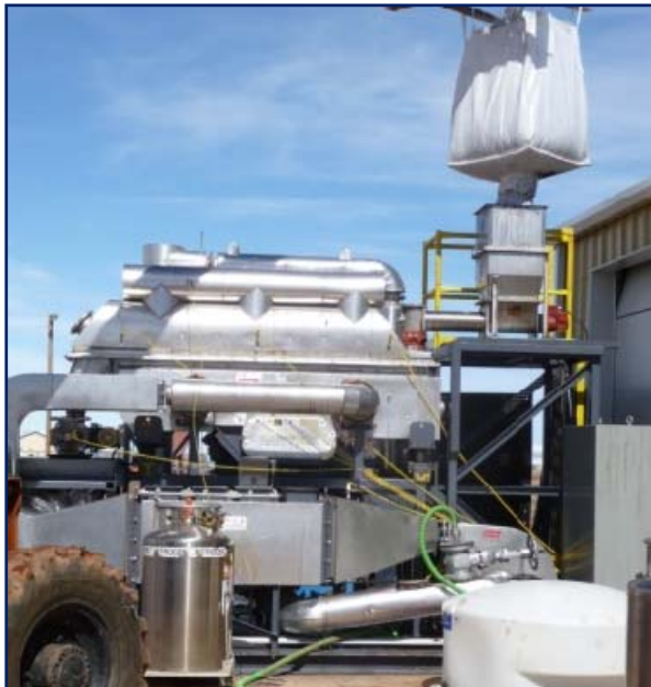
Figure ES-2 Mobile WRITECoal™ 1-2 MW th -Scale Pilot Plant at WRI's Advanced Technology Center.
