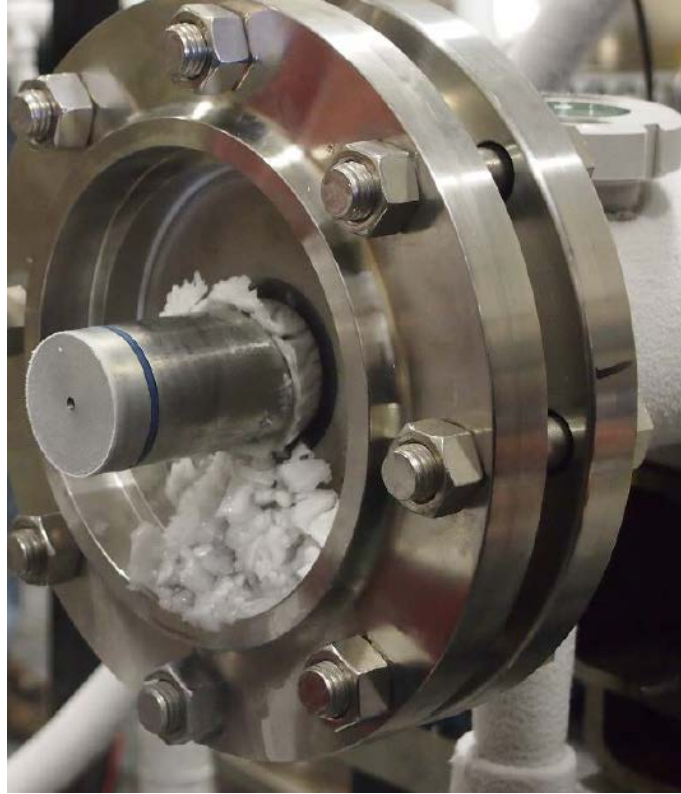
Figure 6. CO 2 solid is extruded from the auger filter during testing.
