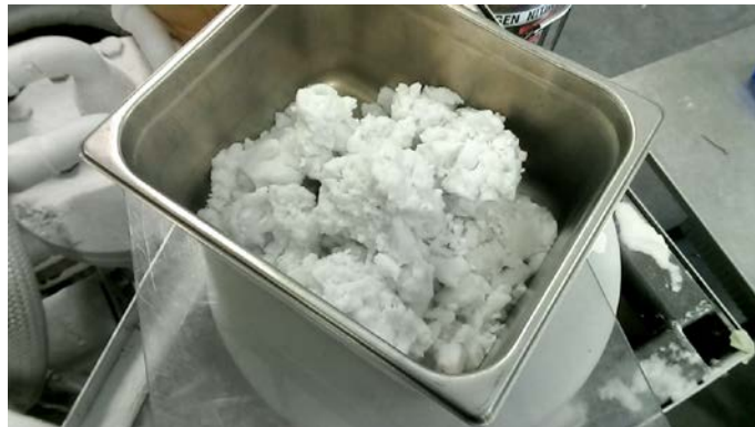
Figure 7. Solid CO 2 captured and separated during testing of the skid-scale system.
