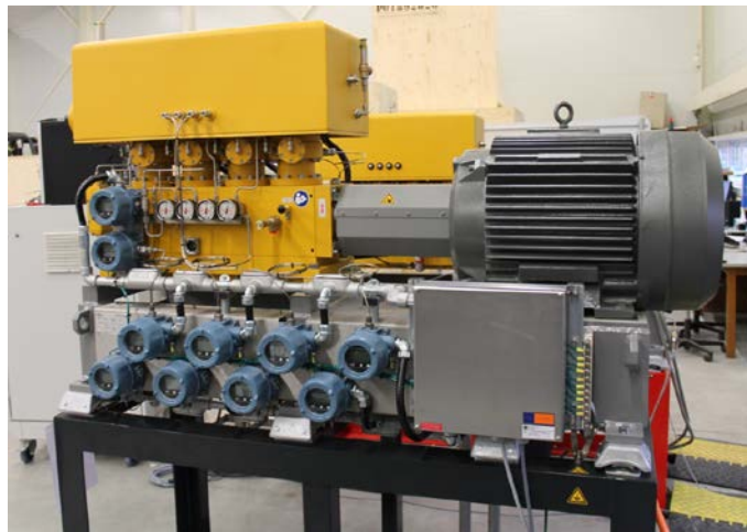
Figure 4. Stirling SPC-4 cryogenerator used to provide all lower-temperature cooling in the ECL skid.
