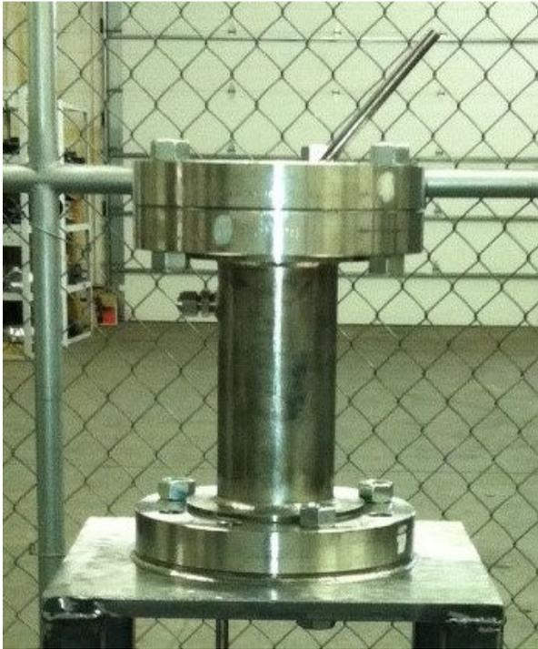
**Figure IV:** *Helical Channel Reactor*
