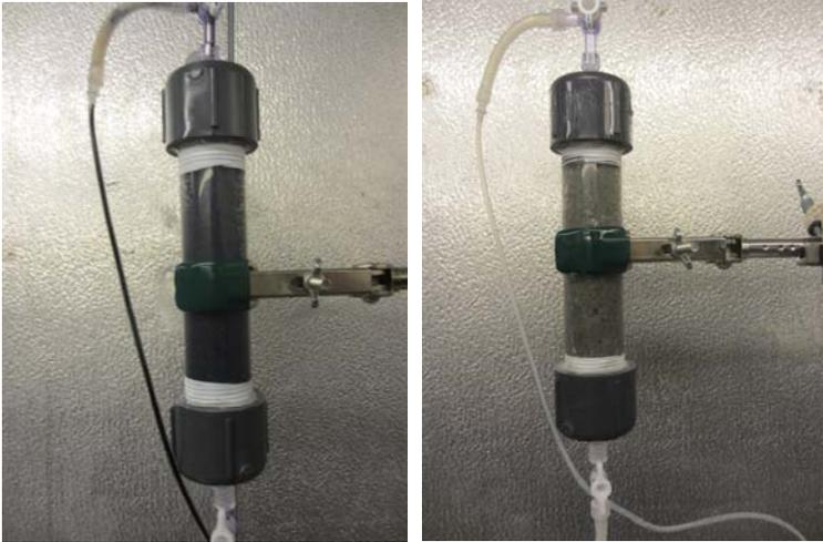
Figures 4 & 5. Visualization of the observable differences between columns in which a reducing environment is suspected to have been created (left) versus one in which little reduction has been demonstrated to have taken place (right). Note the color changes of the tubing as well, which was demonstrated to be sediment and not discoloration by wash out during upgradient water treatment.
