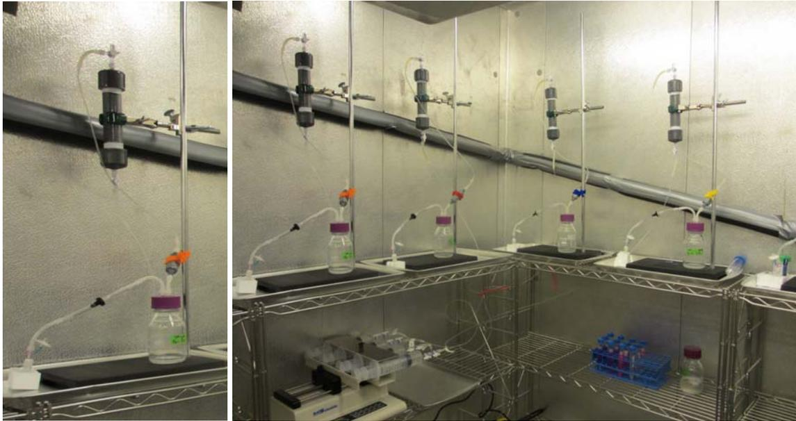
Figures 1 & 2. Pictures of one column and sampling bottle setup along with a view of a four column block attached to a single syringe pump.
