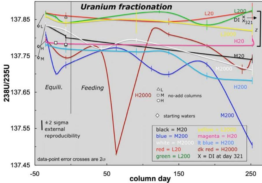
Figure 6.  $^{238}\text{U}/^{235}\text{U}$  ratio values. A designation of a 2 sigma U error bar size is included on the left side of the graph. The bracket on the right side of the graph designates the naturally-occurring  $^{238}\text{U}/^{235}\text{U}$  ratio range determined utilizing zircon (Hiess *et al.*, 2012). Abbreviations: Low TDS/U water (L), Medium TDS/U water (M), High TDS/U water (H), Tryptone stimulation level noted by their number in mg/L.
