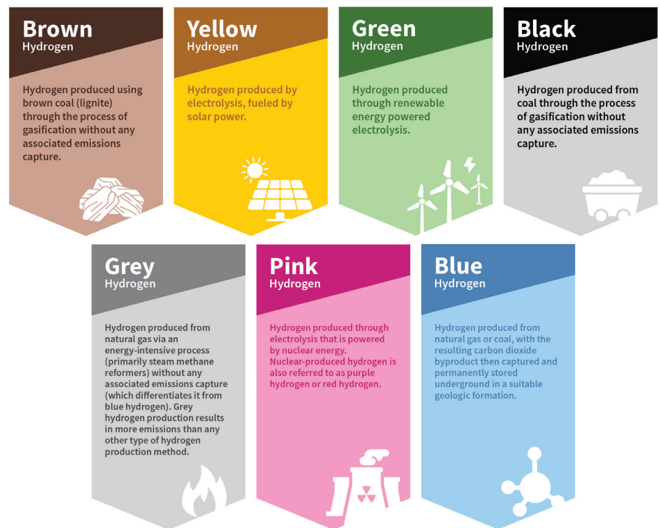
Figure 2: A non-exhaustive depiction of the hydrogen rainbow. As new production pathways develop, they are assigned new colors in the spectrum.
