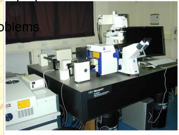
Laser scanning confocal microscope
