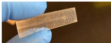
Figure 6: Later rendition of PET lateral flow immunoassay device.
