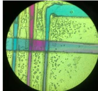
Figure 1: Laser cut Nanoprecipitation device mixing area.
