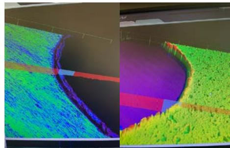
Figure 7: Imperfection (lip) produced by fabrication processes.
