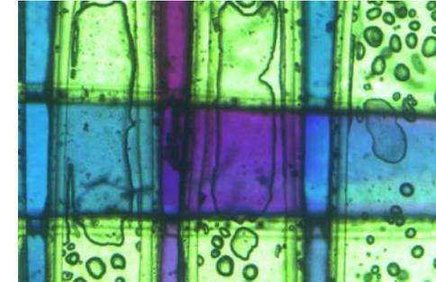
Figure 3: Close of mixing area in laser cut Nanoprecipitation device.
