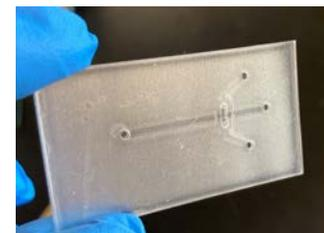
Figure 11: Assembled Nanoprecipitation device.
