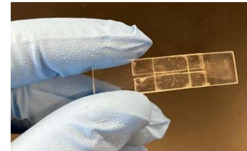
Figure 5: PET Lateral flow immunoassay prototype.
