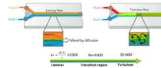
Figure 2: Laminar vs. Turbulent mixing. Credit: Researchgate.com
