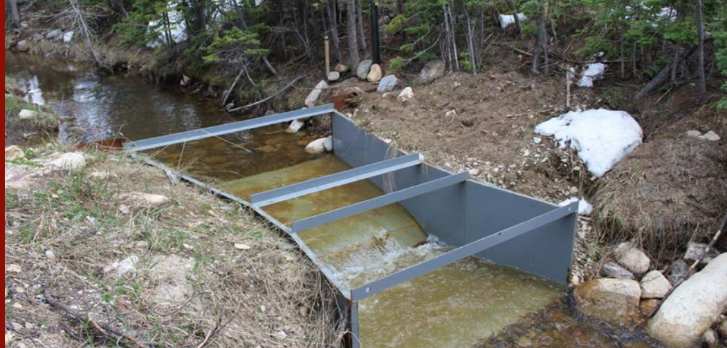
Flumes equipped with telemetry devices (in background) allow for low upkeep, real-time flow monitoring. Photo by Joe Cook.
