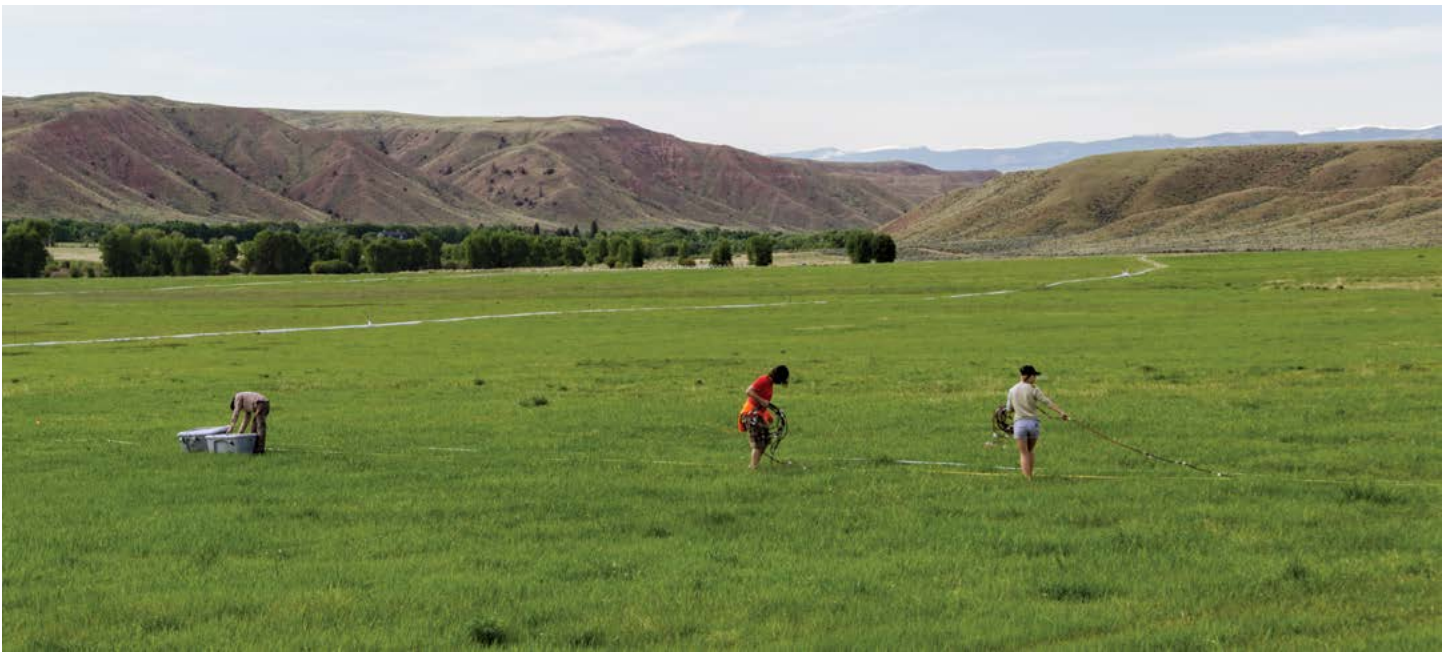
The time-lapse electrical resistivity tomography (ERT) equipment is laid out in a field in the Bear Creek Study area. ERT measures the electrical current (resistivity) in the subsurface using electrodes installed on the soil surface.
