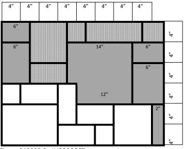
Figure 040000-2: INCORRECT Notching of stone is not permitted. Vertical stones used and 4" increment is not maintained.
