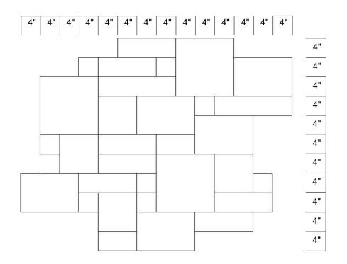
Figure 040000-3: CORRECT Random ashlar pattern with no vertical stones in 4" increments.
