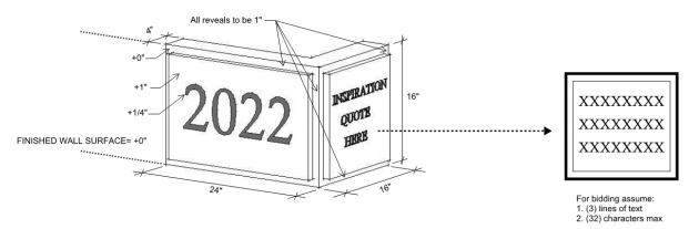
Cornerstones shall be placed on the right corner of the main building elevation with the date facing the main elevation.
