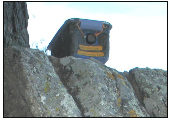
Figure 2: Anabat unit set at the base of Devil's Tower
