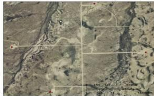
F. High density field (Estimated EI = 0.99 , Approx. 0.25 km between structures, 10 structures per km^2 )
