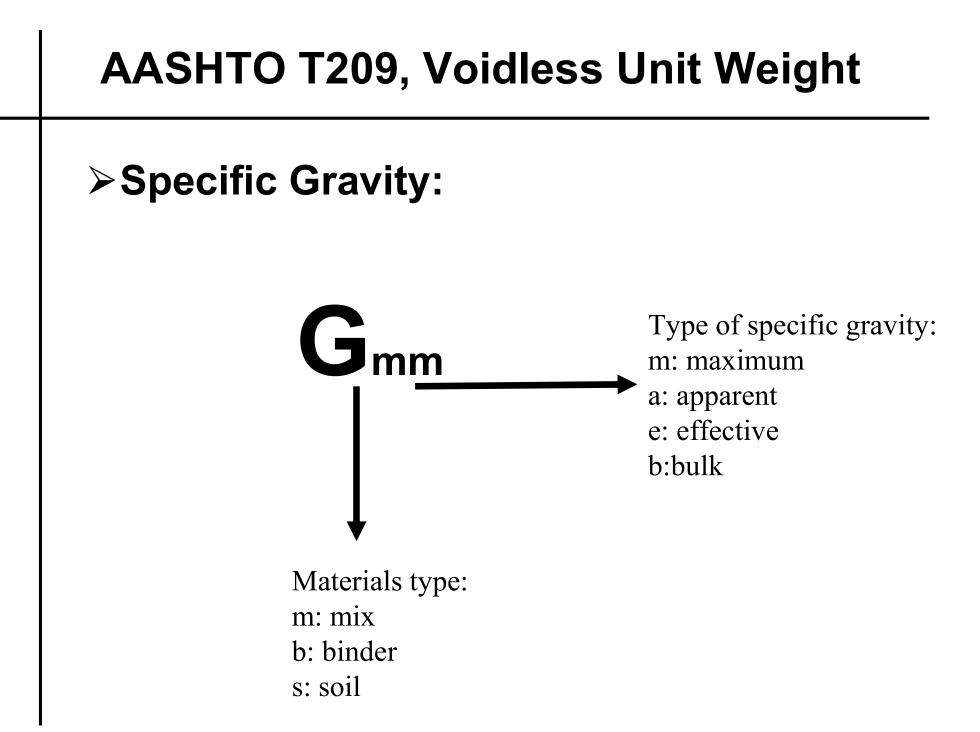
This procedure describes the verification and adjustment of the production mix Voidless Unit Weight (VUW). The VUW is sometimes referred to as maximum density, theoretical maximum weight, maximum specific gravity (Gmm), or Rice specific gravity. VUW for construction mix is conducted under controlled condition.
